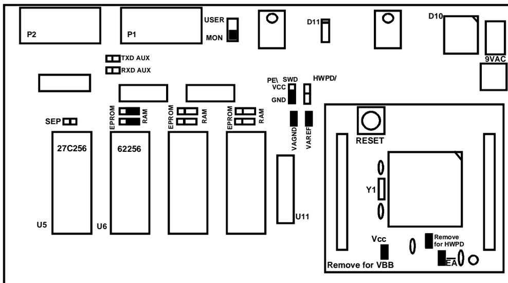
**Figure 2.1 Default Jumper Settings with the 80C535 Processor**
