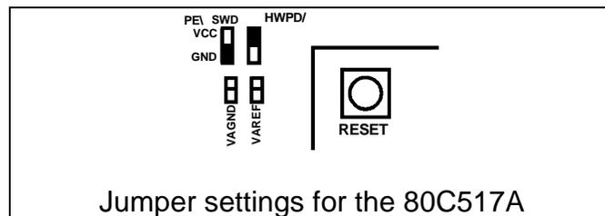
The other pin assignment differences, namely the VBB/VCC pin 37 of the 80535 family and the OWE input of the 80537 family of microcontrollers are addressed by jumpers on the respective daughter boards.
