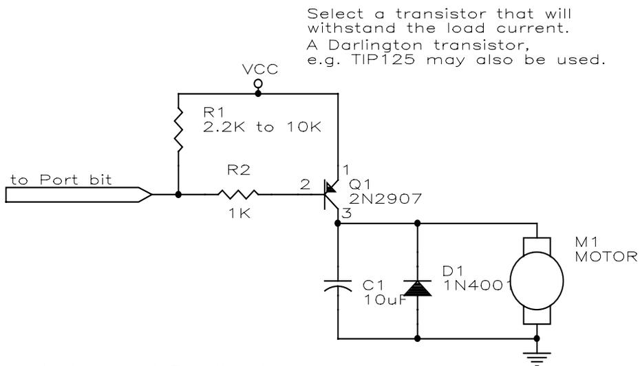
Select a transistor that will withstand the load current. A Darlington transistor, e.g. TIP125 may also be used.
