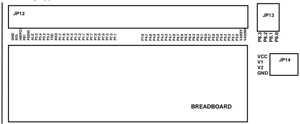
Figure 7.2 JP12, Microcontroller Ports
