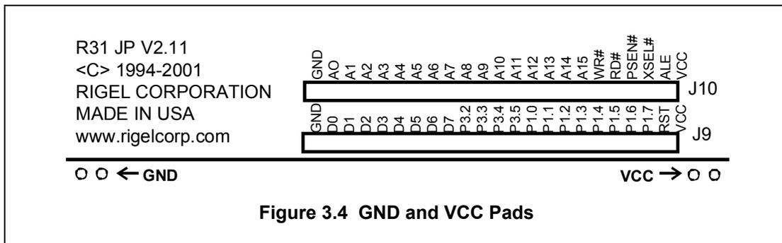
Figure 3.4 GND and VCC Pads
