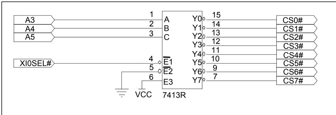
**Figure 9.2 Decoding the Memory-Mapped I/O Space for Eight Devices.**
