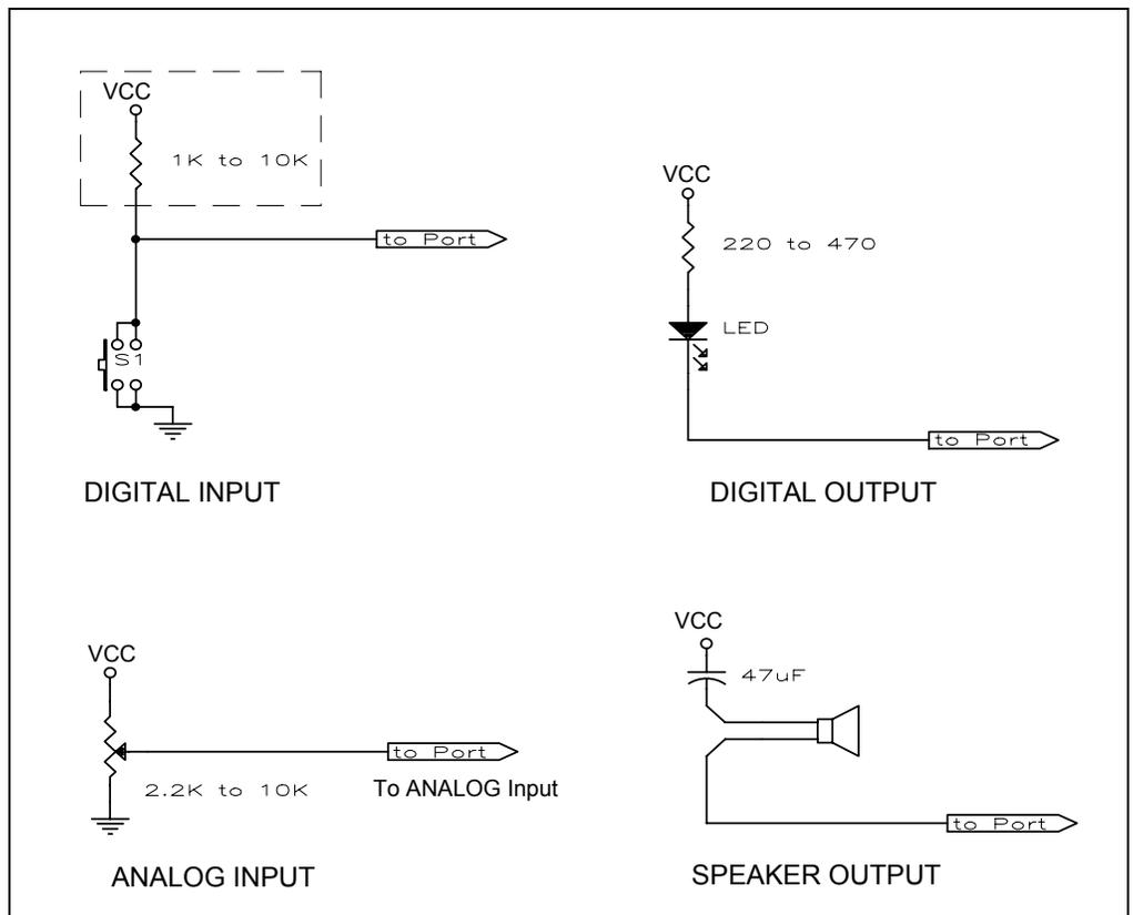
**Figure 9.3 Simple User Input/Output Devices.**
