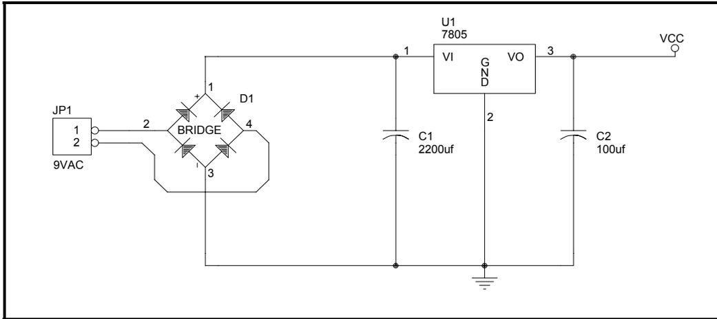
**Figure 1 A Simple Voltage Regulator**
