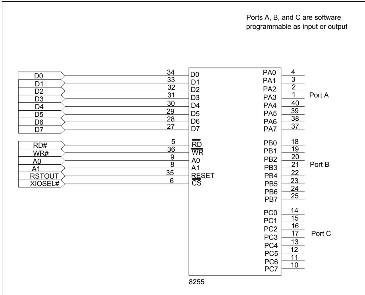
**Figure 9.1 Adding Memory-Mapped I/O ports to the R-31JP**
