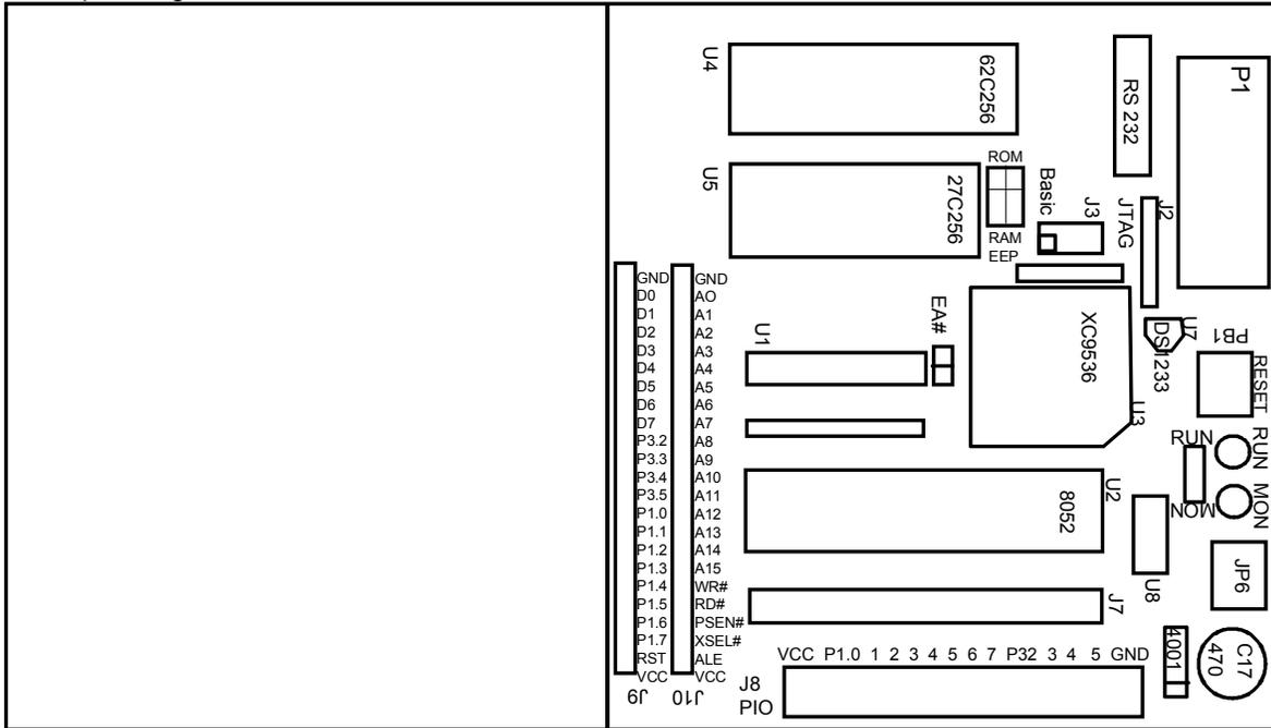
Figure 3.1 Top Board Overlay
