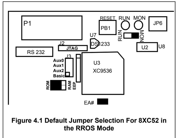
Figure 4.1 Default Jumper Selection For 8XC52 in the RROS Mode
