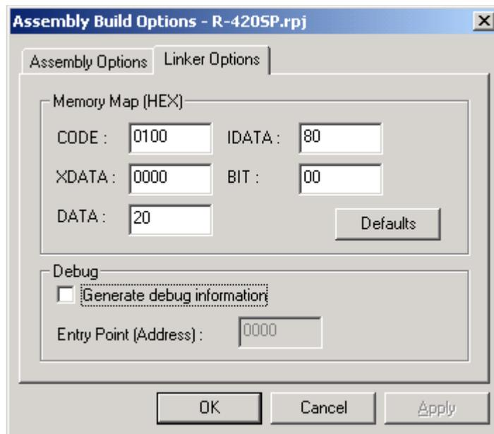
Include a start-up module in your project. This module must be named "c0.src." Enable the internal XDATA RAM in the start-up code. That is, set the PMR (0xC4) to 1. The project R-420SP shows the compiler and linker settings. It also includes the start-up code.
