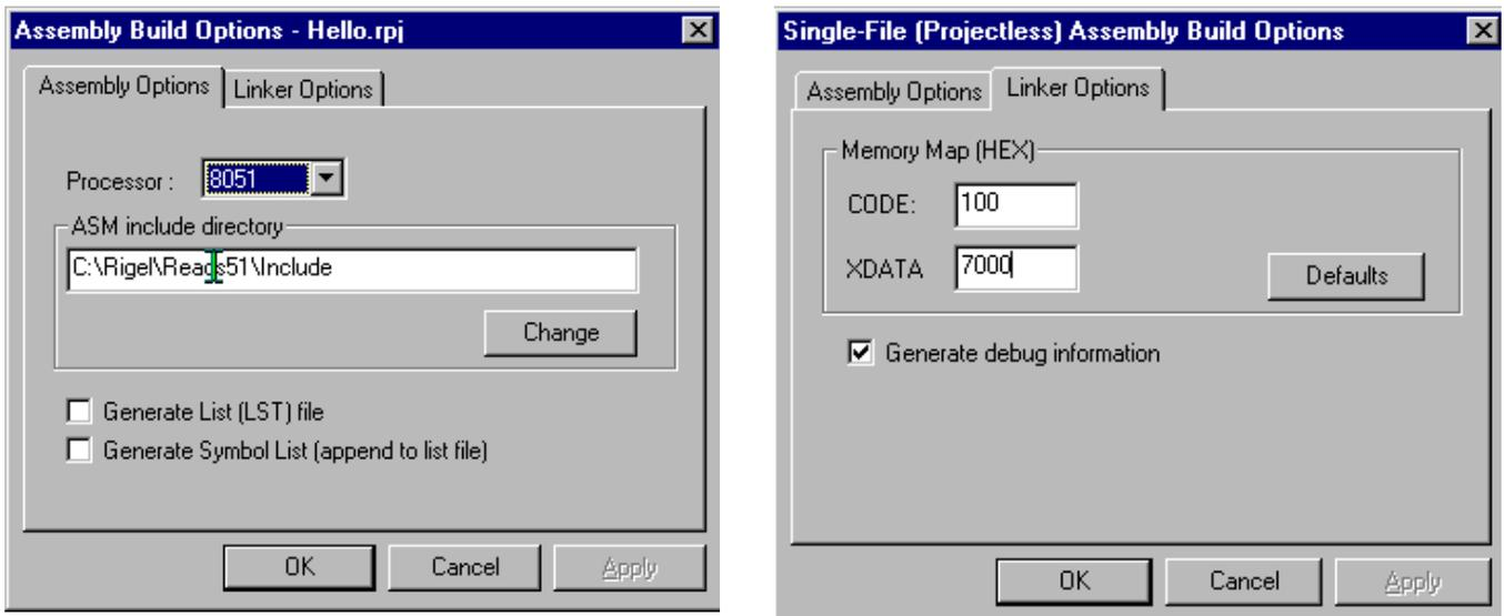
1. The “Generate debug information” box must be checked if you want to debug the code in the Reads51 environment. Please note that currently Reads51 only supports low-level debugging. That is, single stepping, etc. are supported only at the assembly level.
